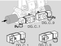
$\rightarrow$  When retrofitting the pressure switch for gas, see enclosed operating instructions "Pressure switches for gas DG..C", section entitled "Mounting the DG..C.. on valVario gas solenoid valves".
