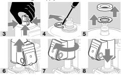
→ In both connection boxes, push through the knock-out for the cable gland set – then remove the covers. The covers must not be taken off before pushing through the knock-outs as it prevents damage to the connection boxes.
