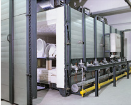
Intermittent shuttle kiln in the ceramics industry
