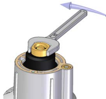
Figure 11 Adjusting flow rate.
