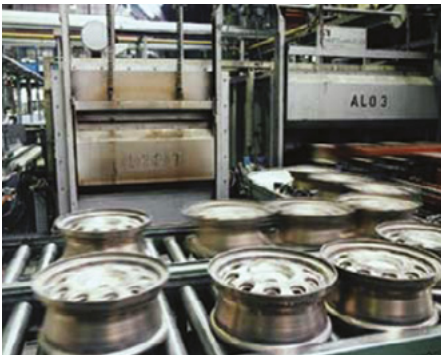
Aluminium industry: curing oven for wheel rims
